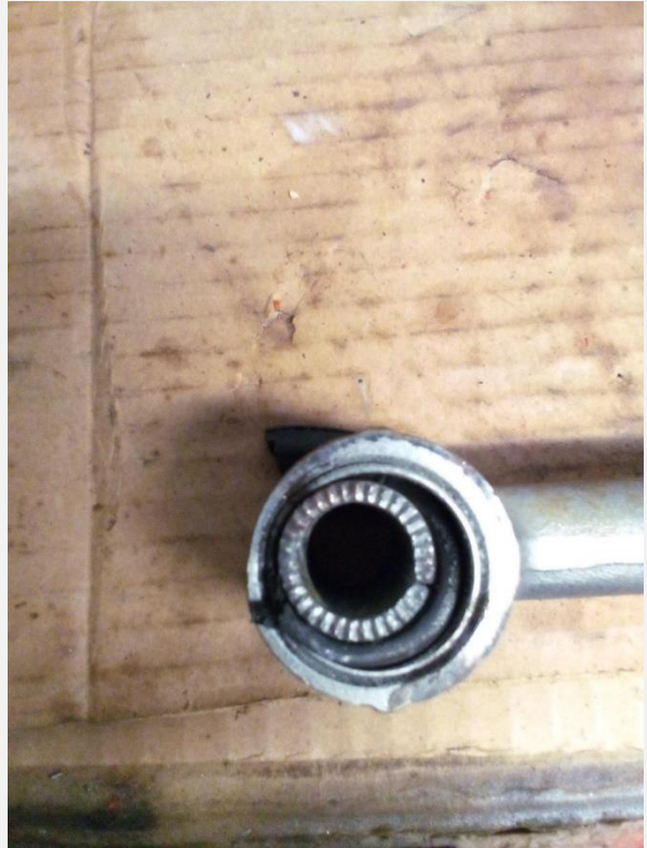
Inner rod strut end worn bushing
