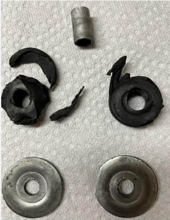
Destroyed steering rod end bushings
