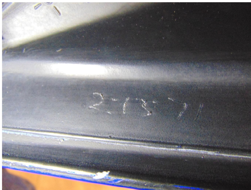
Here is an etching from a 1995. The hood was etched on December 12th and contains a sequence number of 78. Note the formation of the numeral 8.
