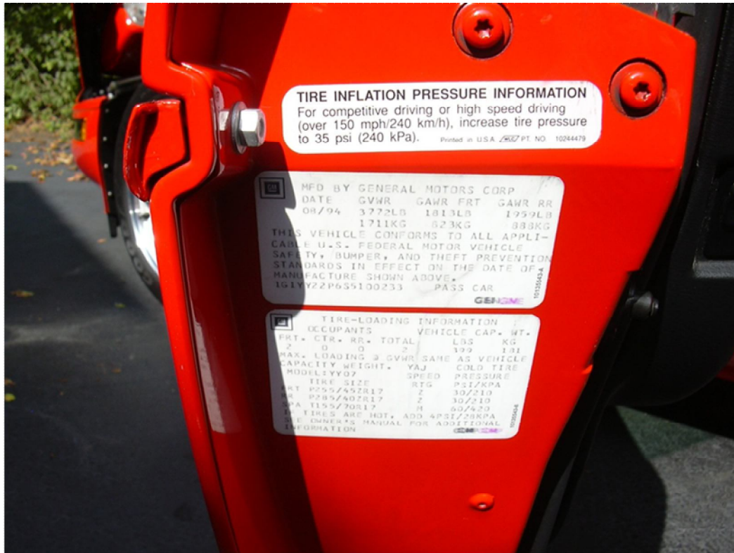
Two examples of previous versions of door jamb labeling
