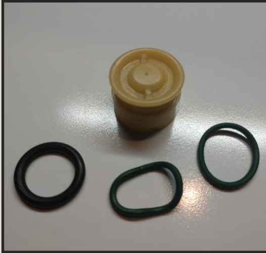
Figure 6 ORIGINAL PISTON W/O-RINGS USED IN 1995
