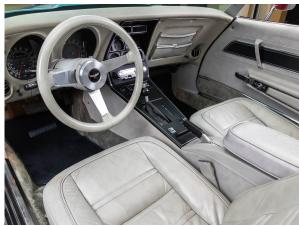
The third photo (smoked grey interior) is an early 1977 that shows the first configuration of the horn button and telescopic lock ring. Note that the horn button is brushed aluminum while the lock ring is the same color as the steering column.
