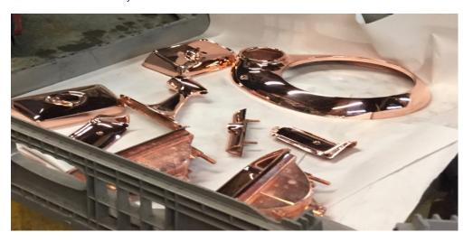
We were shown the front-end grill and accessories for a classic Studebaker in mid process (above), a motorcycle gas tank in a near final process, and bumpers and external accessories for a 1955 Corvette at the beginning of the Chroming process (below).
