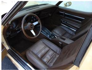
steering wheel center hubs which fail to conform to Federal Motor Vehicle Safety Standard No. 107, 'Reflecting Surfaces'. The horn button cap and the lock lever have a brushed chrome finish. The surface reflectivity of this finish on some of these horn button caps and lock levers is approximately twice the maximum reflectivity allowed by the standard."
