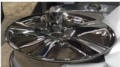
bumpers are already chromed, then the old chrome and any other layers need to be taken off first. And once the basic metal piece to be chromed is prepared, then the chemical processes begin, and there are a number of variables that need to be managed, such as what under layers are desired or needed, such as nickel and copper, and how thick they should be prior to the final layer of chromium.
