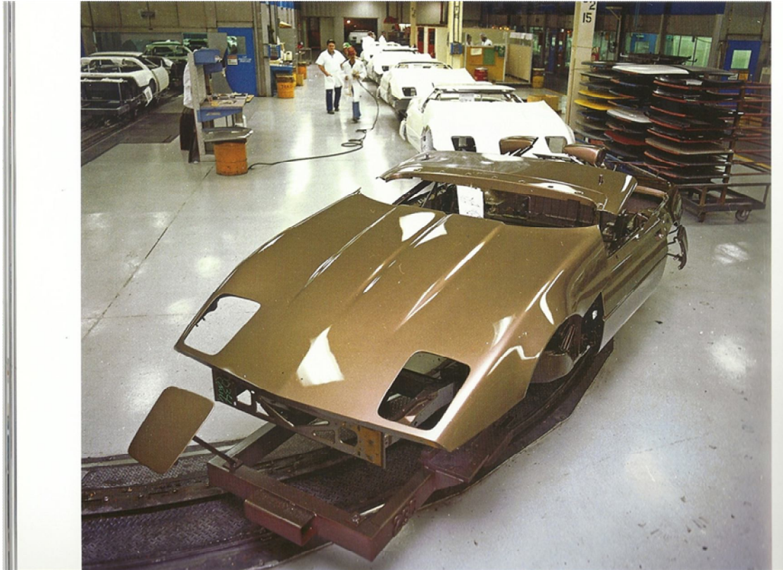
Note the body color on the frame rails and front cross member prior to blacking out
